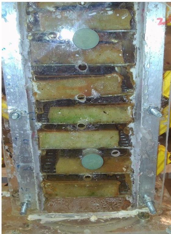
Figure B.3 Growth of algae in SBTF_{CANON} reactor around sponges plate
