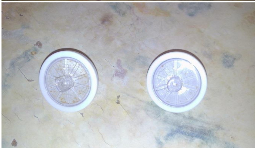
Figure 3.8 1 Biomass collected in SBTF ANAMMOX reactor during sampling (syringe). b) Biomass retained in the filters after filtration (left side) SBTF ANAMMOX and SBTF CANON (right side).
