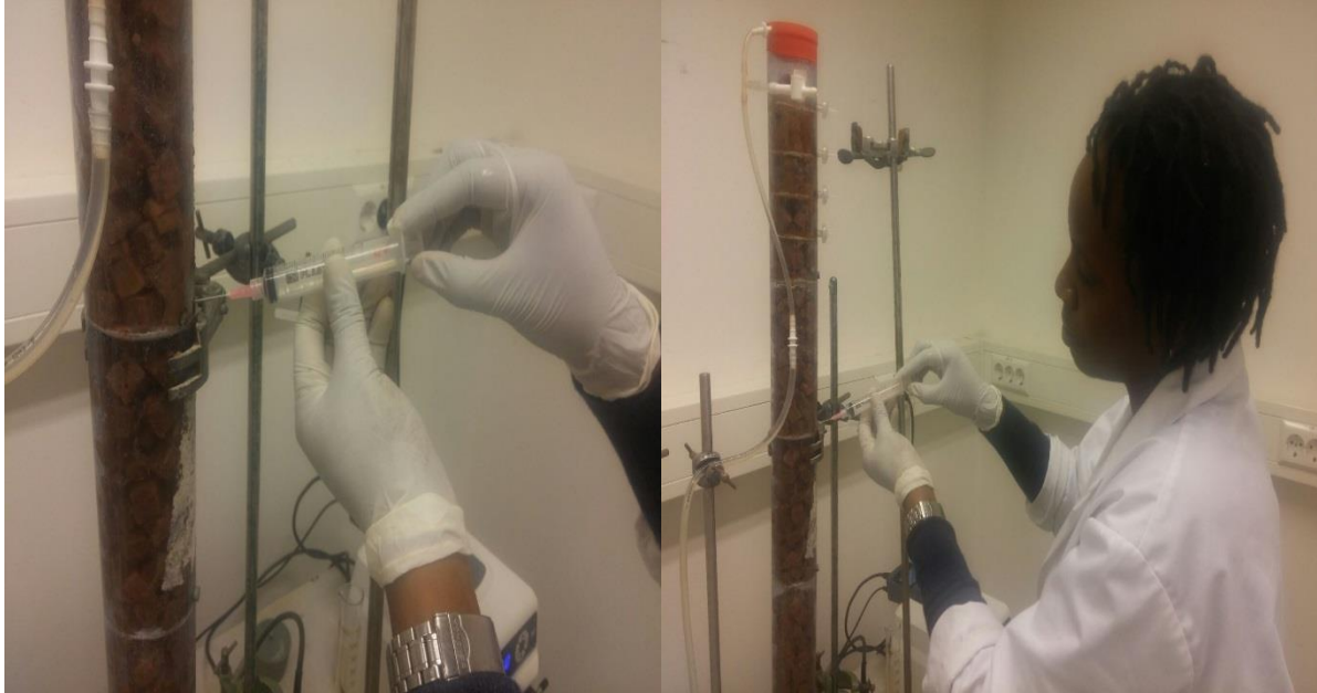
Figure 3.6. 1 Sample collection in SBT FANAMMOX reactor compartments
