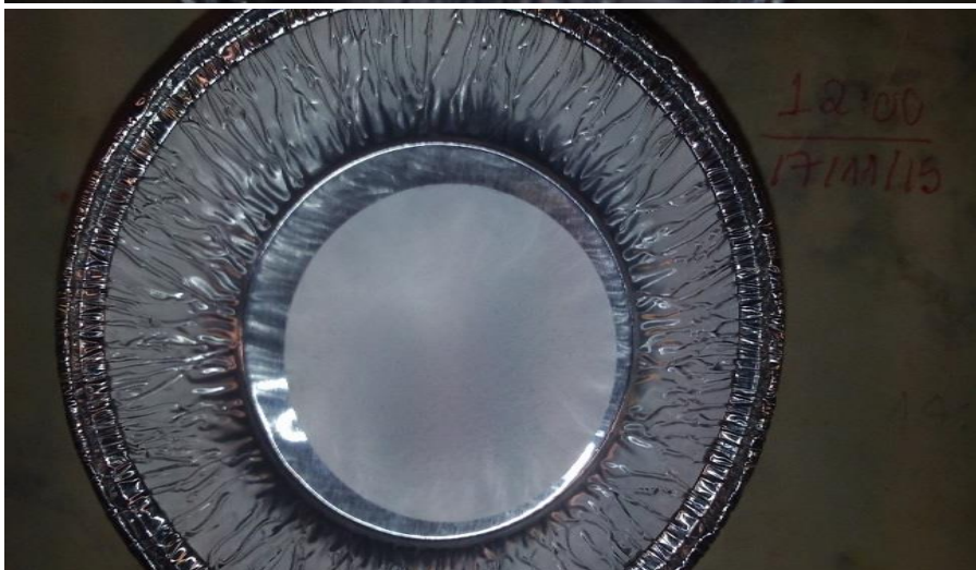
Figure 3.11. 1 Biomass retained in the filters before TSS and VSS measurement. a) Sample from SBTF ANAMMOX reactor. b) Sample from SBTF CANON reactor.
