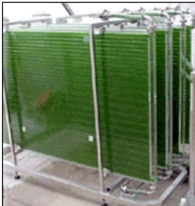
Figure 2-21 Flat plate photobioreactors, from (Ojamäe, 2011)
