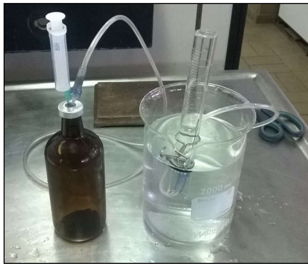
Figure 3-12 Tightness test on the biogas measuring system
