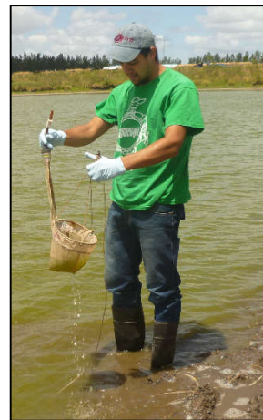
Figures 5-11 Draining water from the phytoplankton net after dragging it with the rope from inside the water
