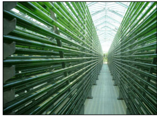
Figure 2-20 Tubular reactors. Left: pilot scale (own picture). Right: prototype scale from (Ojamäe, 2011)
