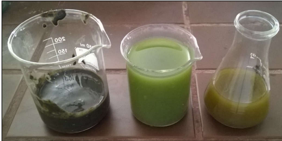
Figure 3-4 Biological materials, from left to right: anaerobic inoculum, cyanobacteria, wastewater
