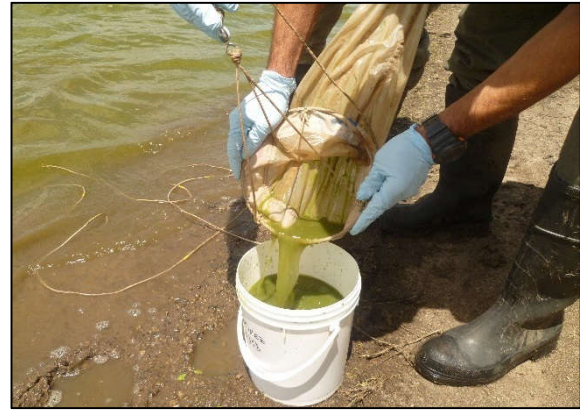
Figures 5-10 Harvesting cyanobacteria with rope. Left: throwing the net. Right: transferring the filtrate to a bucket.
