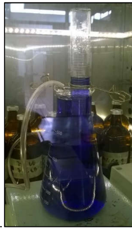
Figures 3-16 Wet chemistry biogas analysis: adding NaOH into the measuring liquid
