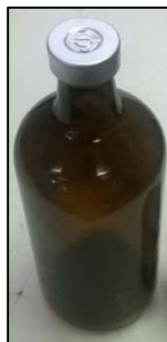
Figure 3-6 Left: Glass opaque amber 500 mL bottles. Right: 30 mm aluminium cap and butyl rubber seal
