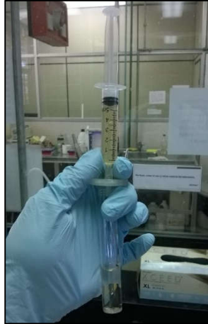
Figures 3-19 Filtering resultant licqour of BMP tests.
