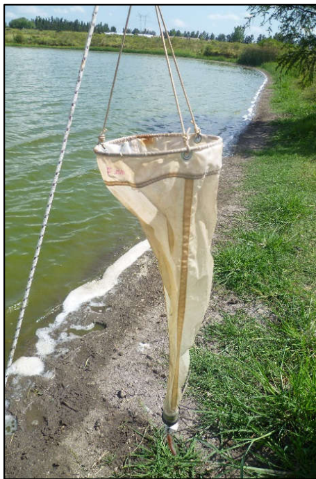
Figure 3-3 Phytoplankton net of 0.25 \mu\text{m} of pore opening.
