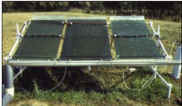
Figure 2-21 Flat plate photobioreactors, from (Ojamäe, 2011)
