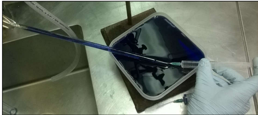
Figures 3-17 Wet chemistry biogas analysis. Left: displacing a basic solution. Right: measuring the headspace.
