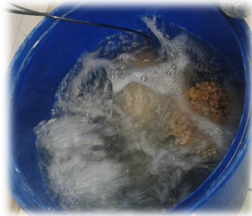
Figure 18: Membranes submerged into a tank with Citric Acid for chemical cleaning
