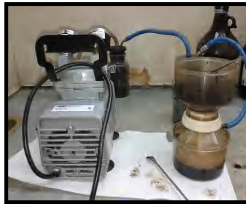
Plate A7. Coal slurry product / Vacuum filtration
