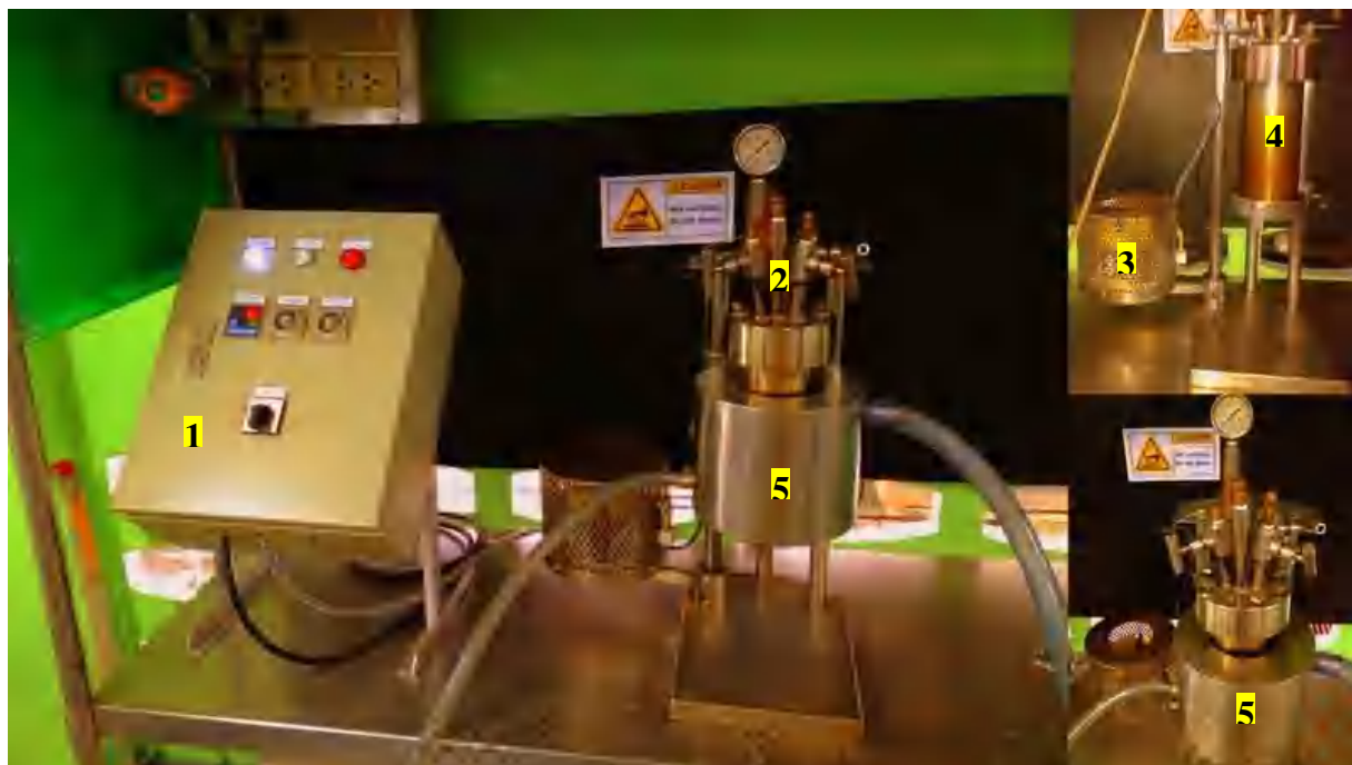
Figure 3.2 Laboratory setup of HTC reactor
