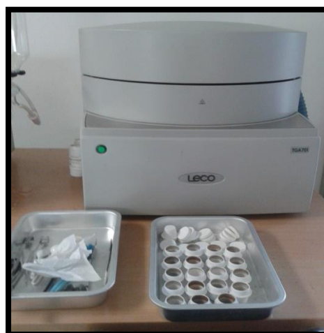
Plate A4. Bomb calorimeter and Thermo gravimetric analyzer (Leco, USA)
