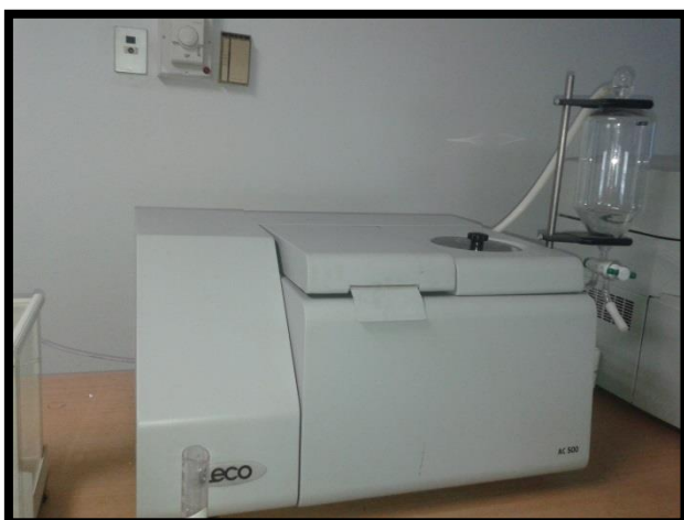
Plate A4. Bomb calorimeter and Thermo gravimetric analyzer (Leco, USA)
