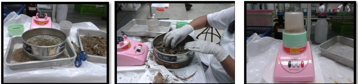
Plate A3. Preparation of samples (cutting/chopping/sieving/grinding)
