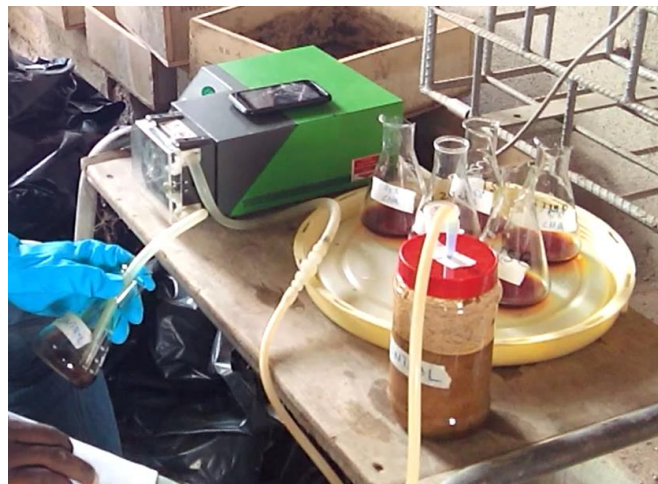
Plate 3-11: Set up of peristaltic pump for siphoning of gas from headspace of sample
