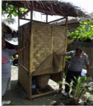
Single-vault UDDT in Libertad, Misamis Oriental, Philippines [Source: www.sswm.info ].
