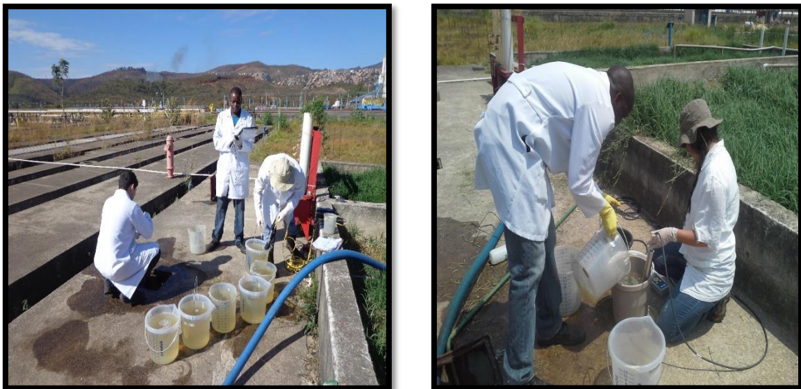
Figure 4.17: Measurement of the effluent outflow and TSS concentration over time.
