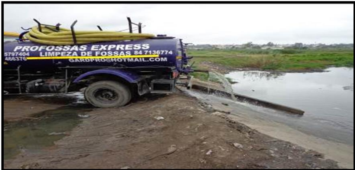
Figure 1.2. Truck discharges content of septic tank sludge from households to stabilization pond in Maputo.
