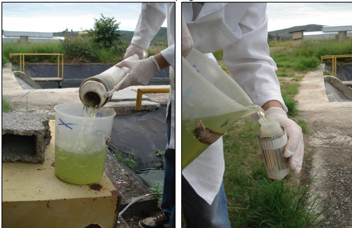
Figure 5.9 - Pouring the effluent from the core sampler into beaker and recipient after sampling.
