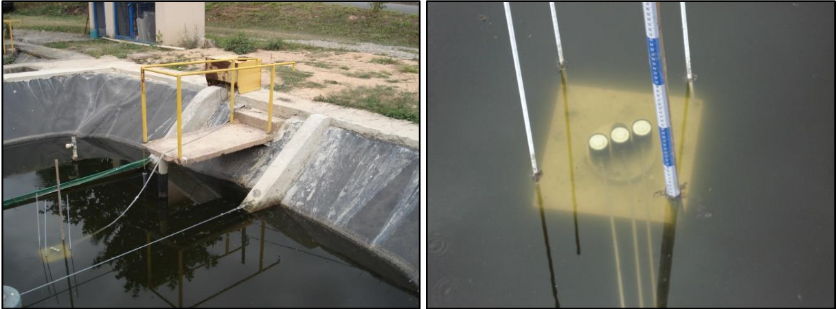
Figure 5.13 - UV-A, UV-B and PAR sensors placed at P_2B_3 at 0.05 m in depth for continuous monitoring over one week.
