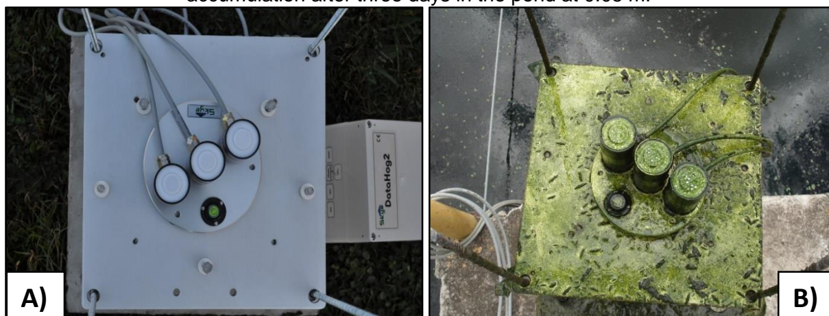
Figure 5.15 - (A) Clean sensors before placed in the pond; (B) Algal and biofilm accumulation after three days in the pond at 0.05 m.
